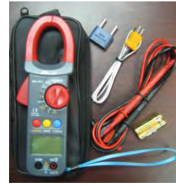
MA-823 DIGITAL CLAMP-ON METER WITH TEMPERATURE
