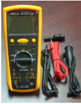
MA-12700A MEGOHMMETER AUTO-RANGING INSULATION TESTER
